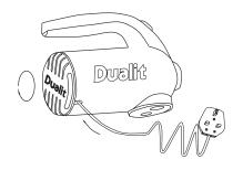
• To prevent cord damage always pull power cord (5) out gently. If the cord jams, rotate the swivel base (4) counter clockwise half a turn, then pull out the cord (5)
