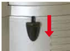
Release the coffee grinder by lowering the lever and twisting it several times. Switch the appliance back on.
