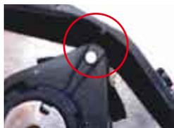
From underneath the unit, check the alignment of the plastic tooth with the reference marks on the bushing. These must be perfectly aligned.
