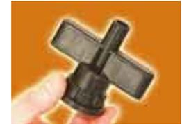
Insert the spanner in the rubber bushing.
