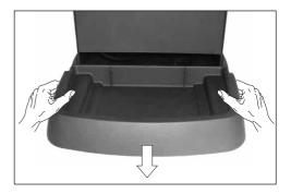
Filter holder and filter: use a moistened cloth and rinse the filter holder with filter inserted with hot water after each use. Once a month take out the filter from the filter holder (with the help of a spoon handle) and rinse it with hot water.
