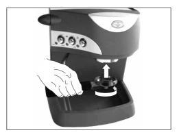
Turn on the machine (as described in the paragraph above) and wait until the heating-temperature light 4 goes off (about two minutes). (It is normal if some water drips out of the filter holder)
